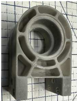
Left – 3D printed Prototype of the wrist joint, printed on a FormLabs 2 SLA Printer
