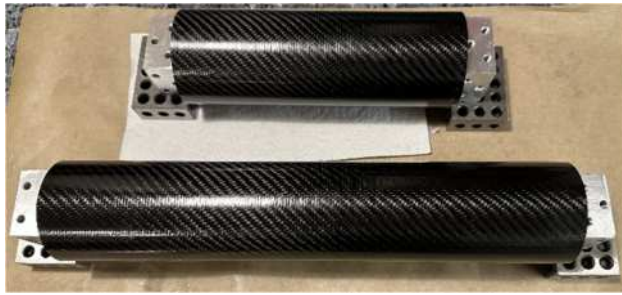
Left – Final carbon fiber arm links after final glue up
